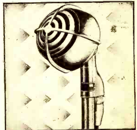
CARDIOID CRYSTAL-LABYRINTH MICROPHONE The Shure "Uniplax" 730-A is a diaphragm-type unit with uni-directional cardioid characteristics (obtained through the addition of an acoustical labyrinth).
